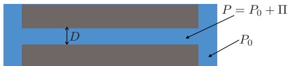
Figure 1.4: The disjoining pressure between two parallel surfaces, where P is the pressure in the film, and P_0 is the pressure of the bulk phase. This figure is a modified sketch from (Butt et al., 2003).
