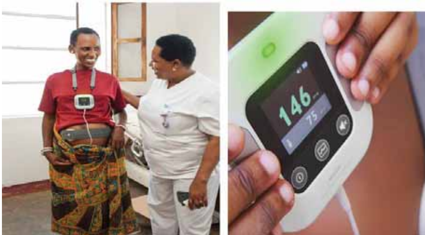
Photo 4: Part 1: Moyo sensor strapped onto the mother's abdomen for prolonged monitoring. Lightweight and portable, it allows the mother to move around freely. Part 2: Metal pads to detect maternal heart rate (Photo reprinted with permission from Laerdal Global Health)
