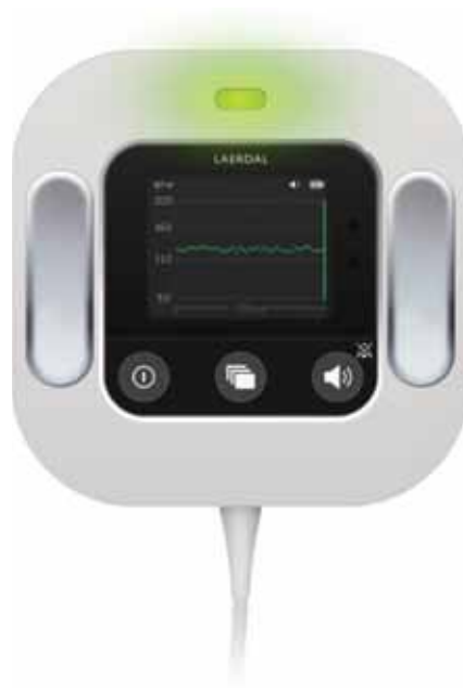
Figure 2. The Moyo FHR monitor with a 30-minutes historical display (Laerdal Global Health).
