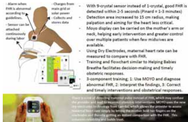
Fig 1. Moyo—The new continuous fetal heart rate monitor (Laerdal Global Health). FHR abnormalities defined as absent, FHR<120 or FHR>160bpm).
