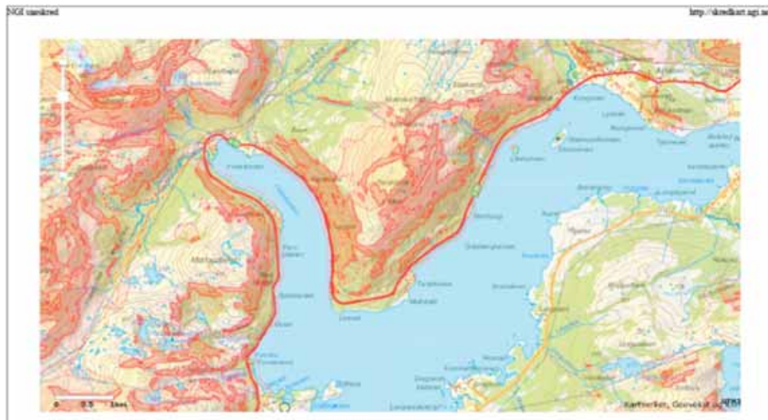
Fig. 3. Example of open source avalanche map of Lødingen, Nordland, North-Norway, provided by NGL. The dark red delineated area represents avalanche release areas (inclinations steeper than 30°). The pink delineated area represents theoretical maximum runout zones. (For interpretation of the references to colour in this figure legend, the reader is referred to the web version of this article.)
