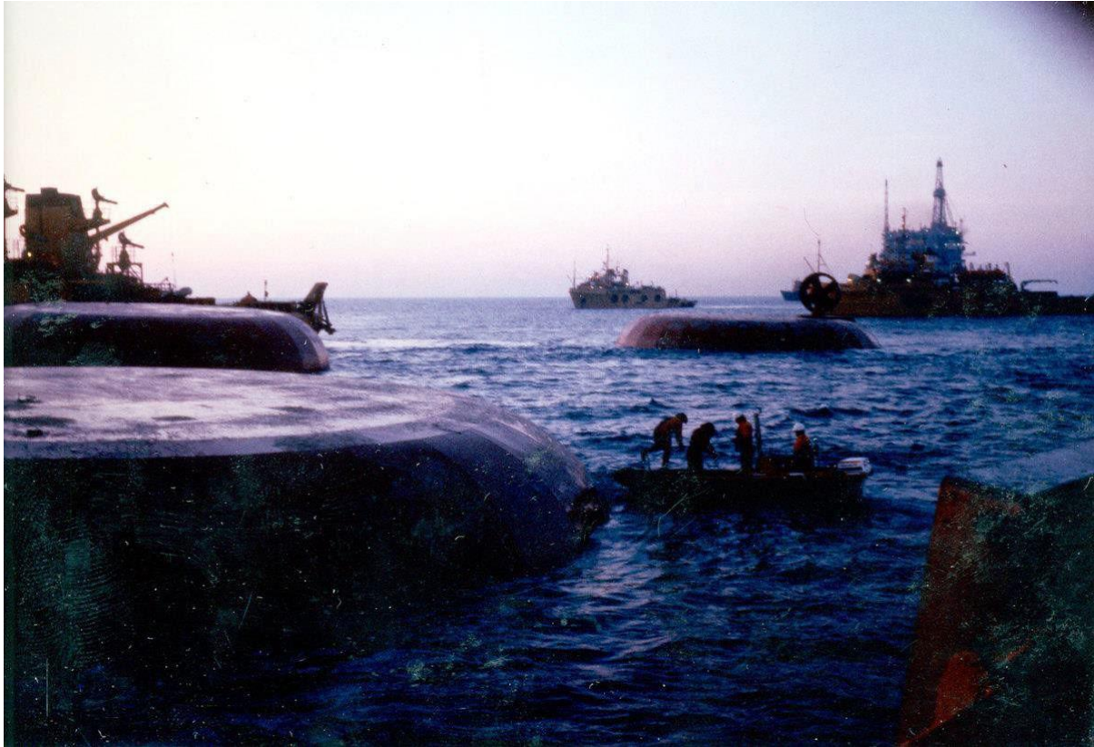
Photo 2. In this photo, three out of four pontoons are visible. The men in the boat are presumably preparing to attach ropes to tow Alexander L. Kielland from Ekofisk to the mainland. The vessel on the left side is the Seaway Falcon. The vessel on the right side is the Wildrake. Photo: Torger Berge/Norwegian Oil Museum. Used with permission.
