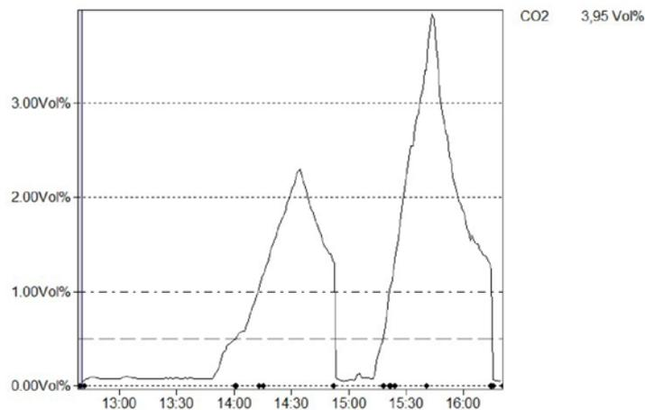
Figure 4: CO<sub>2</sub> build-up (percentage of CO<sub>2</sub>) in the air inside the lifeboat as function of time.
