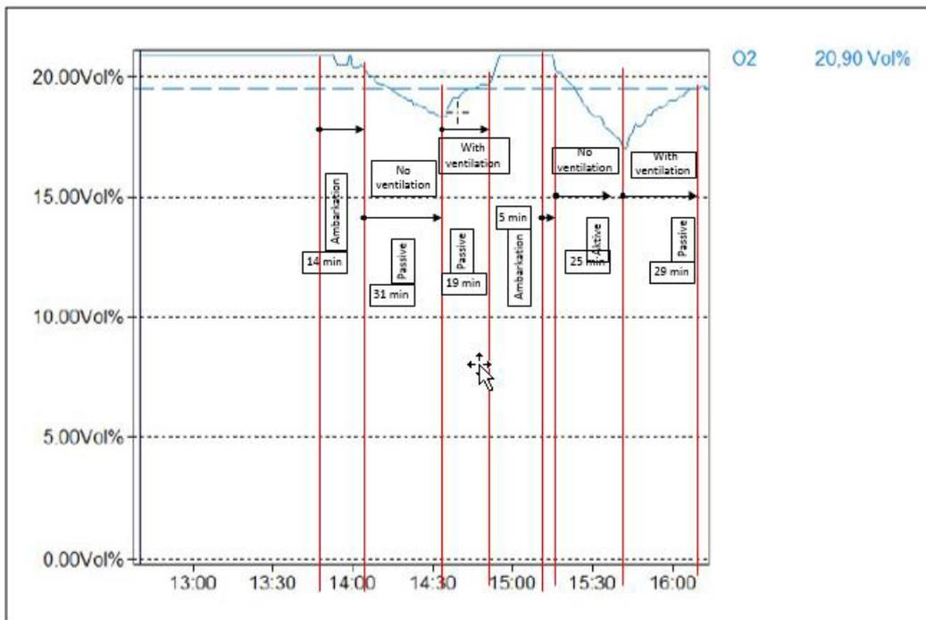
Figure 2a. Volume of O<sub>2</sub> in the lifeboat as function of time with 49 persons onboard.
