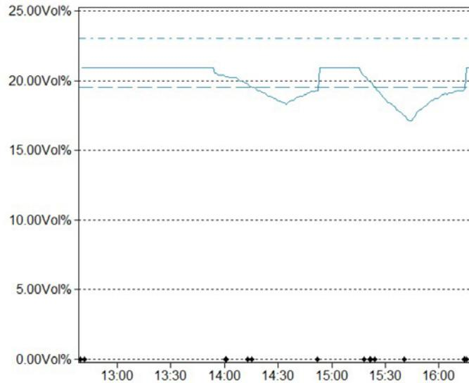
Figure 3: O<sub>2</sub> level (percentage of O<sub>2</sub>) in the air inside the lifeboat. The dashed lines represent the recommended O<sub>2</sub> level.
