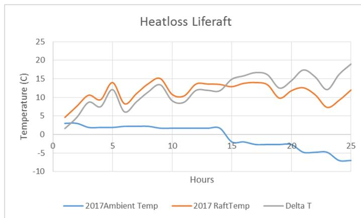
Figure 12 Heat loss in life raft
