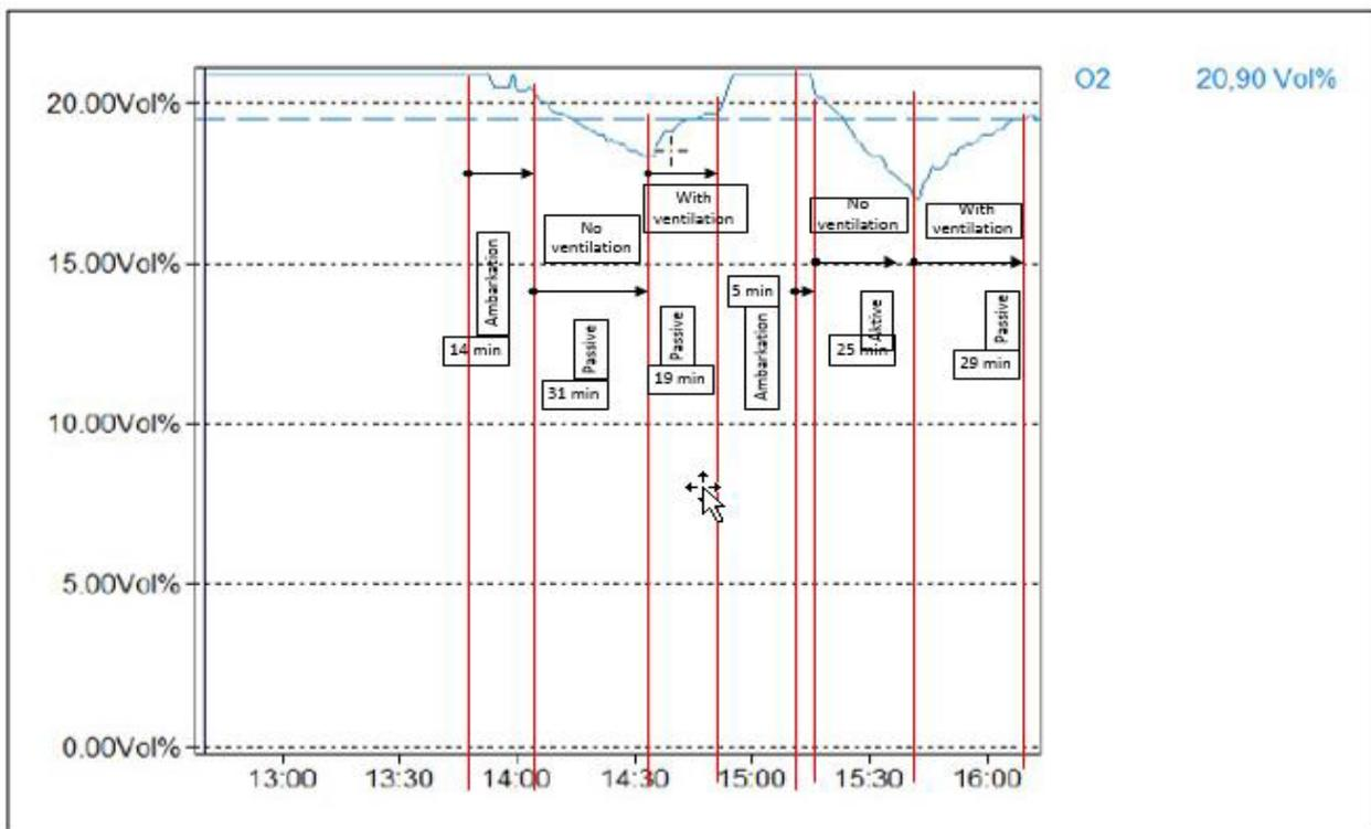
Diagram 2 (Air quality and ventilation test)
