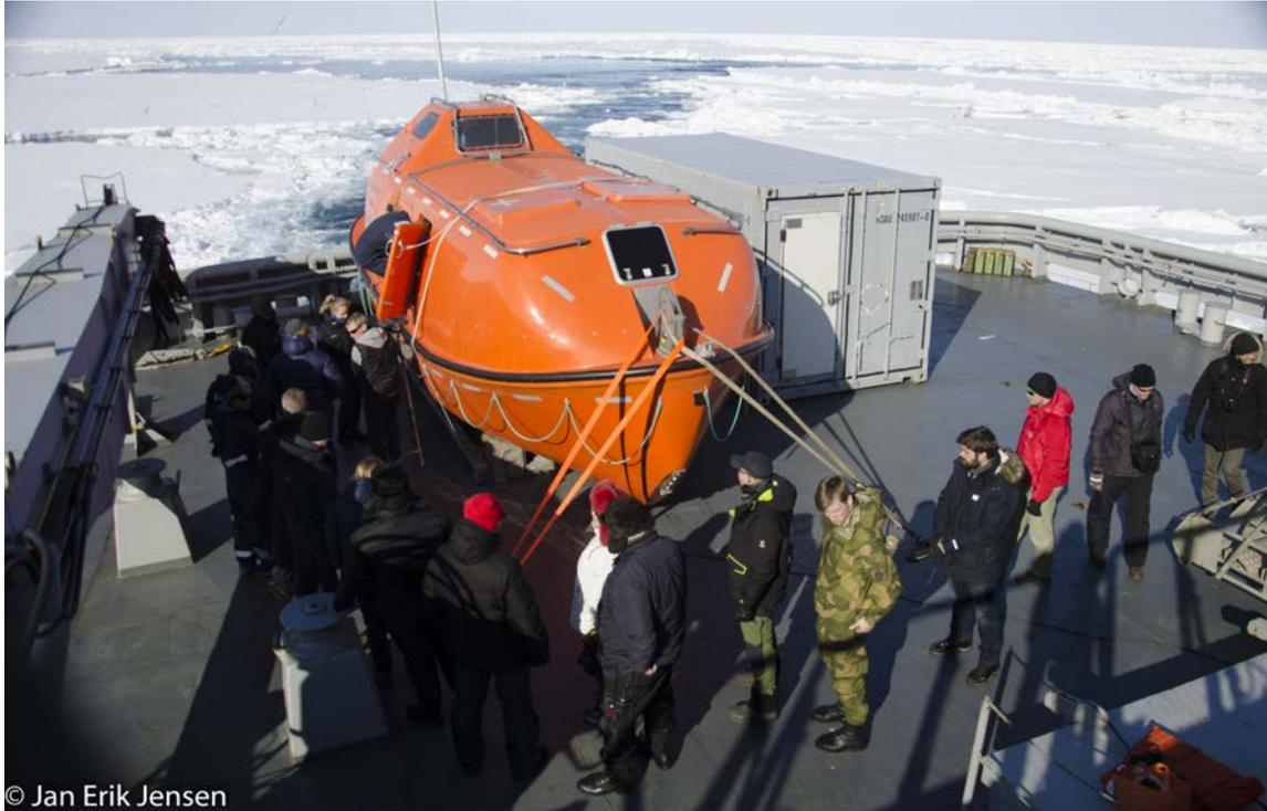
Boarding of lifeboat for O<sub>2</sub>/CO<sub>2</sub> tests.
