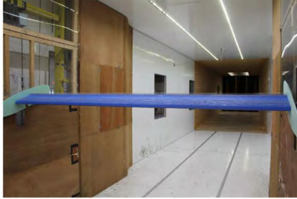
Figure B.1: A view of the Lysefjord Bridge section model during the static wind tunnel tests conducted by SOH Wind Engineering LLC [181].
