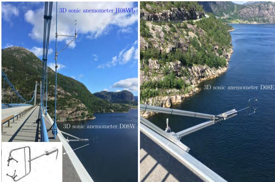
Figure 3.8: A view of the sonic anemometers D08W and H08Wb (left panel) and a close-up on the bracket supporting sonic anemometer D08E (right panel). Photos by N. Daniotti - UiS.
