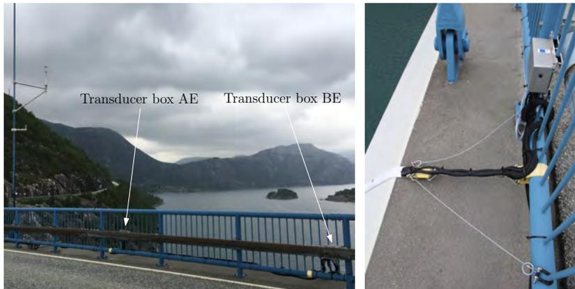
Figure 3.20: A view of two transducer boxes on the east side of the bridge deck (left panel) and a close-up showing their fixture (right panel).
