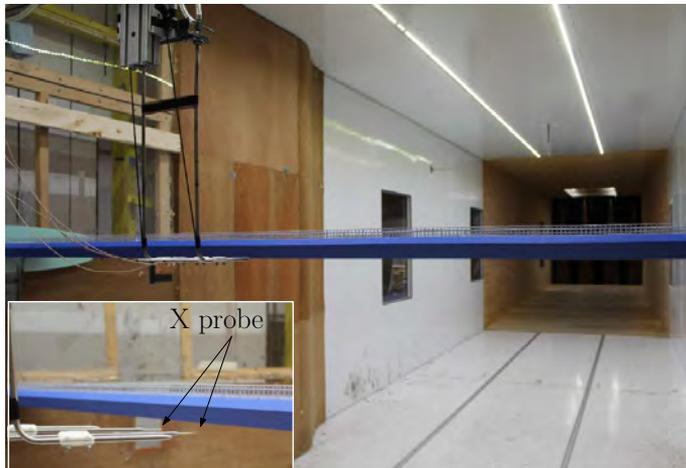
Figure B.6: A view from downstream the section model of the X-probes configuration. The photo is from SOH Wind Engineering LLC [182].
