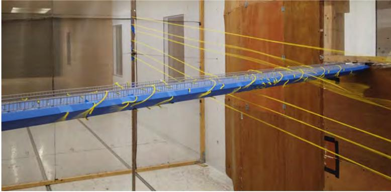
Figure 5.15: A snapshot of the flow visualizations for yawed section model ( $\beta = 25^\circ$ ) in smooth flow, showing a signature of the axial flow in the near wake. The photo is from SOH Wind Engineering LLC [182].
