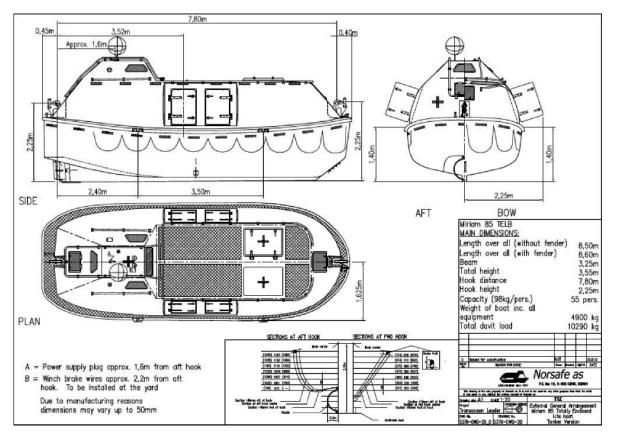
Figure 1. Details of lifeboat used in the exercise
