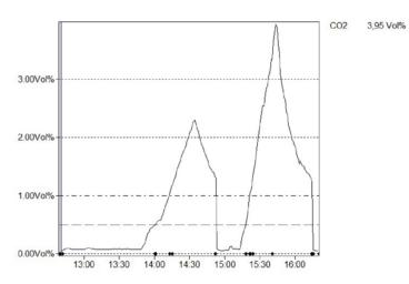
Figure 4:  $CO_2$  build-up (percentage of  $CO_2$ ) in the air inside the lifeboat as function of time.
