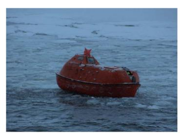
Figure 2: Lifeboat used for exercise 2016 and 2017. (2017: With considerably improved insulation and heating arrangement).
